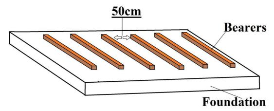
**4.4. Assembling the walls**: place the wall-boards on the bearers as shown in a general sample below:
