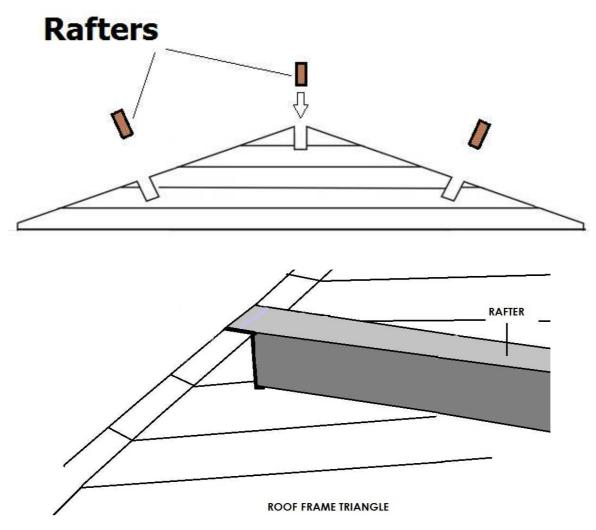
**4.7. Roof-boards:** The next step is to attach the roof-boards vertically and screw them into the rafters. Make sure the ends of the roof-boards are perfectly parallel to each other. Then fix the roof plank boarder under the roof-boards as show below. The roof-plank must be screwed to the roof plank boarder.
