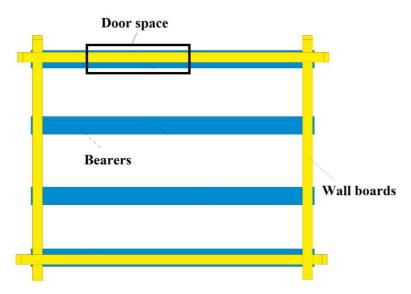
The wall-boards must be placed so that the ends interlock. Now screw the first row of wall-boards into the bearers. All the following rows of placed wall-boards should interlock not only at the ends, but along their length as well. Please screw each new row of wall-boards into the former row to ensure a solid structure.
