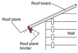
**4.8. Wind-boards:** Place the wind-boards on top of each other to make a 90 degree angle. Now attach these ones on a roof frame triangle and fix with screws.
